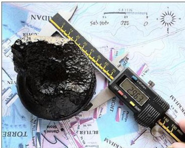
**Read Projectile direct caliper diameter measure of 2.96 inches at bourrelet. Projectile radius (used in ArcCalc) =  $2.96/2=1.48$  inches**
