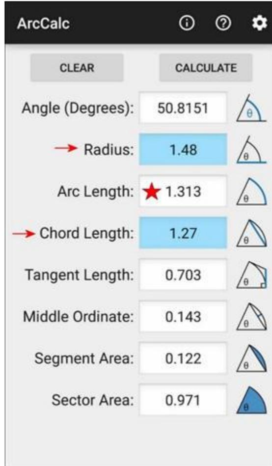
The L+G chord length value (1.27) and the measured radius (2.96/2) can be used in the above equations to obtain the estimated total number of land and groove sets (N) that could be fit around the circumference of the sabot using the calculated L+G arc length (1.313):
