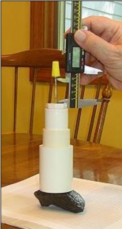
First, place the Plunger on a flat surface and “zero” the caliper between the top of the cap of the Plunger (Part 4) and the base of the washer glued beneath wire nut. Next, remeasure the distance of travel on a shell fragment with the “zeroed” caliper and it will directly read values similar to what is in the above table.
