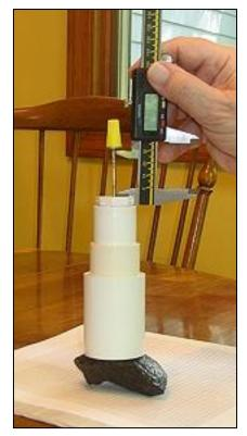
First, place the Plunger on a flat surface and "zero" the caliper between the top of the cap of the Plunger (Part 4) and the base of the washer glued beneath wire nut. Next, remeasure the distance of travel on a shell fragment with the "zeroed" caliper and it will directly read values similar to what is in the above table.
